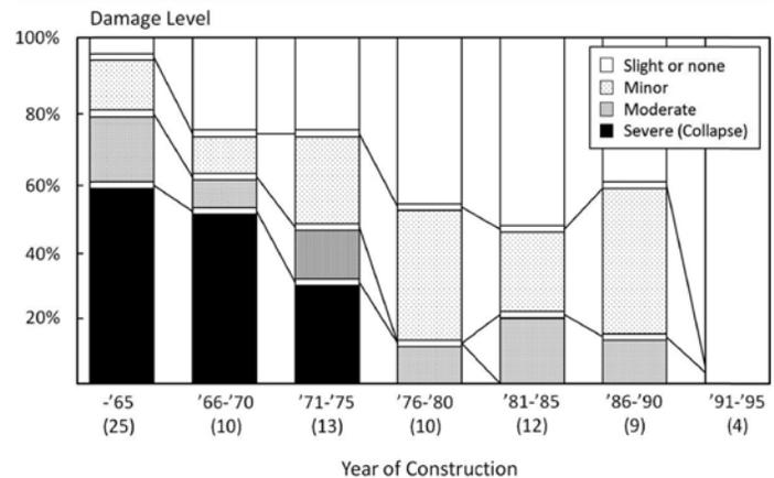
Figure 2. Correlation of damage observed in the 1995 Kobe earthquake with age of structures.
